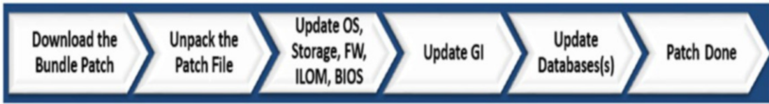
Figure 8-10. Patch cycle of Oracle Database Appliance
